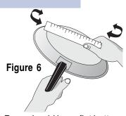
Pans should have flat bottoms. Check for flatness by rotating a ruler across the bottom. There should be no gaps between the pan and ruler.
